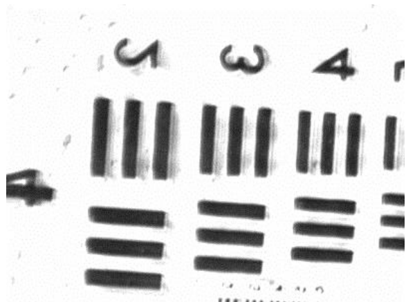
Figure 3 Reflected light image of metal film resolution target.
